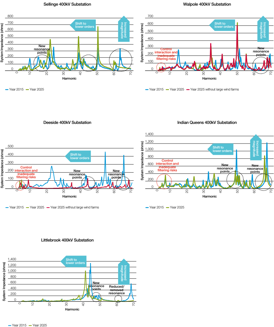
Figure 54 Frequency Scans up to 70th Harmonic Order in 2015 and 2025
